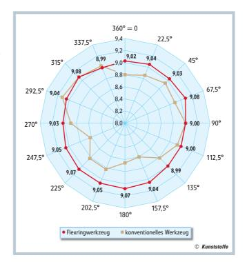
Fig. 3. Wall thickness distribution over the circumference of the die achieved with a Flexring die through local optimization of the flow channel gap (pipe geometry: 110 x 9 mm)
