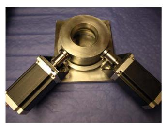
Fig. 1. Exhibition model for demonstrating the benefits of tiling die technology. The four flange bolts are used not only for clamping purposes, but also to tilt the die (photos without fig. 4: Gross)
