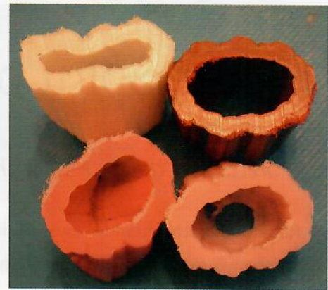
Fig. 7. Color exchange trials: the improved mixer spider-leg system results in uniform colors over the entire cross-section of the samples, which were removed at different times during color exchange trials (© H. Gross)
