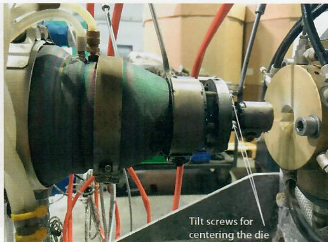
Fig. 4. Tube head with tilt die and axial setting screws during the testing at Siro-Plast GmbH
