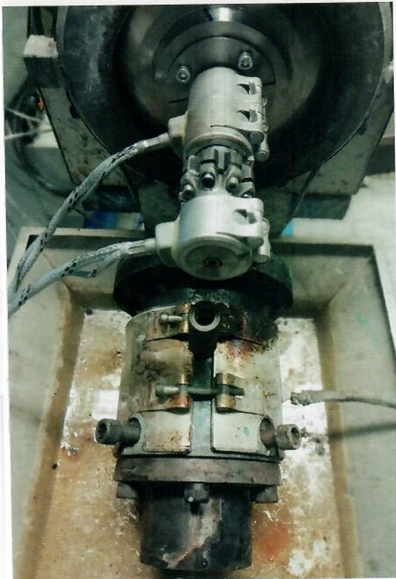
Size comparison: the mixer spider-type head mounted on the extruder, which is manufactured by an additive process, without the heating tapes, weighs 480 g; the conventional head lying below it in the catch basin weighs 820 g.
