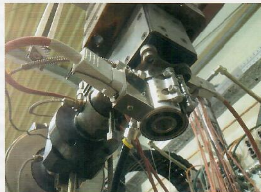
Fig. 5. Mixer-spider-type head with counterrotating spiral mixer spider legs: 3D view (left) and mounted on the trial extruder (right)
