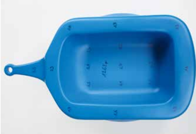
Fig. 1. The weight and wall-thickness distribution (thickness values in mm) of the top side of the trailer manufactured with a conventional conical die (figure: Gross)
