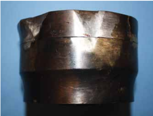
Fig. 3. GWDS mandrel, which has been manually profiled in the end region in an extreme manner in order to improve the wall thickness distribution in the region of the trailer loading platform (figure: BIG)
