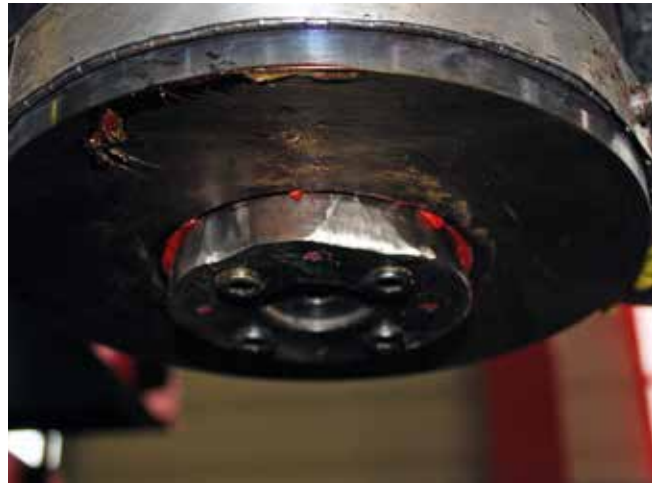
Fig. 4. Mandrel situation in which the melt-flow distribution of the parison is not influenced by the extreme profiling at the mandrel end, since the profiling is outside the flow channel (figure: BIG)
