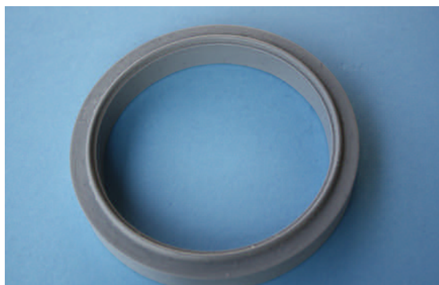
Fig. 1. Seal of the head illustrated in Figure 5 (sustained temperature resistance of 300 °C) with which the gap between the head and the die is sealed and which permits tilting and shifting of the die
