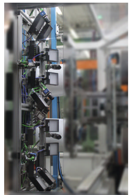
The IMLWatcher inspects the quality of labeling
