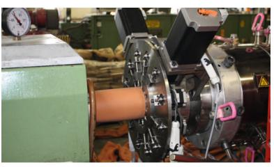
Fig. 5. Flexring tool used for the tilting technique – for the first time, it is thus possible to conduct closed-loop control of eccentric, as well as asymmetric variations in thicknesses
