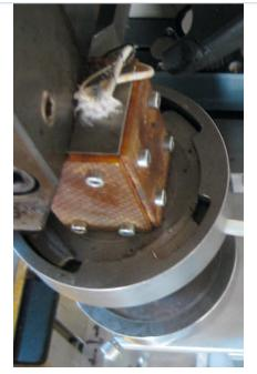
Fig. 3. Bayonet lock coupling of a capillary die with tilting technique
