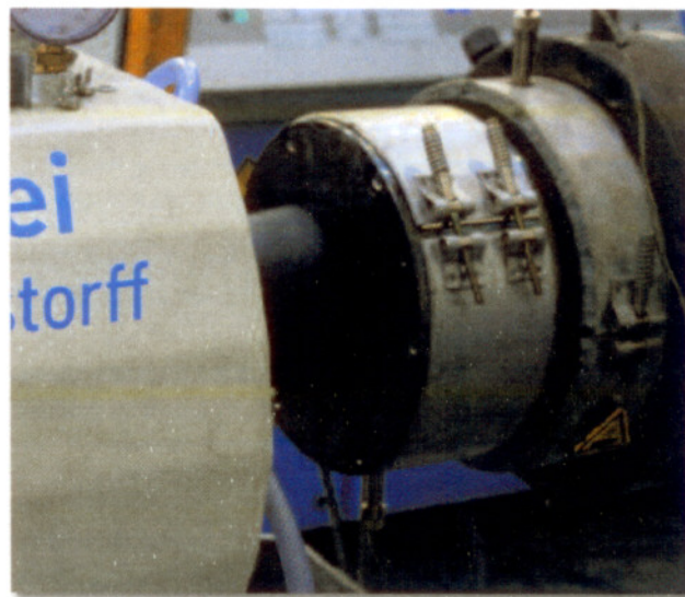
Fig. 3: Pipe head that has been retrofitted with a tilting joint during tests at Krauss Maffei
