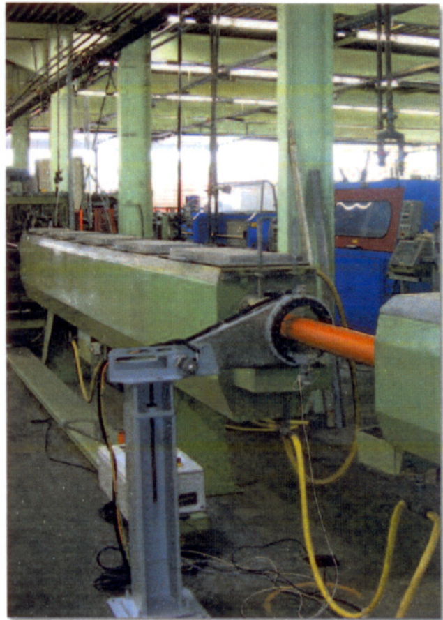
Fig. 6: Pilot system to measure the thickness during tests in a production line for 110 mm of core foamed PVC-pipes
