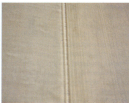
Fig. 2. Comparison of the silhouette of the test films produced in the Chill-Roll process (right half with die lines running in the direction of extrusion) and those with a closed polishing gap (left half without die lines) (photo: Gross)
