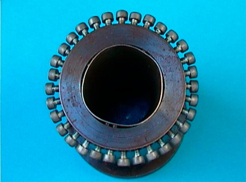
Fig. 2 Flex Ring head having been statically deformed by using adjusting screws
