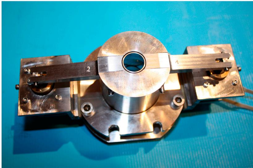
Fig. 3 Flex Ring unit to be retrofitted into a twelve cavity head for the production of an oval bottle having a volume of 200 cm<sup>3</sup>
