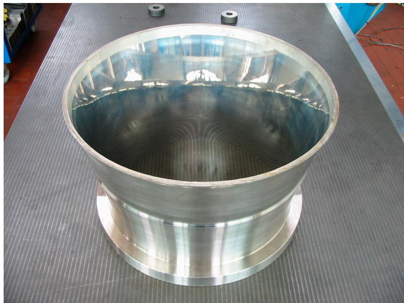
Fig. 1 Flex Ring sleeve for the production of industrial bulk containers (IBC), having a diameter of 550 mm and a flexible multi-walled conical wall which has been retrofitted into an existing head
