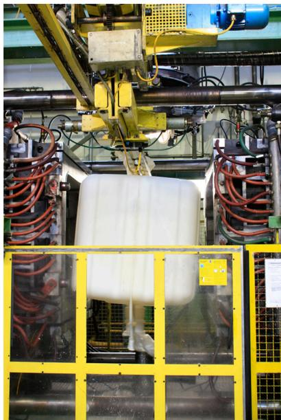
Fig. 7 IBC taken out of the machine at the end of the production cycle
