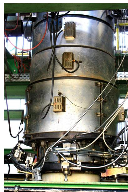
Fig. 9 Complete head with integrated dynamic radial wall thickness control
