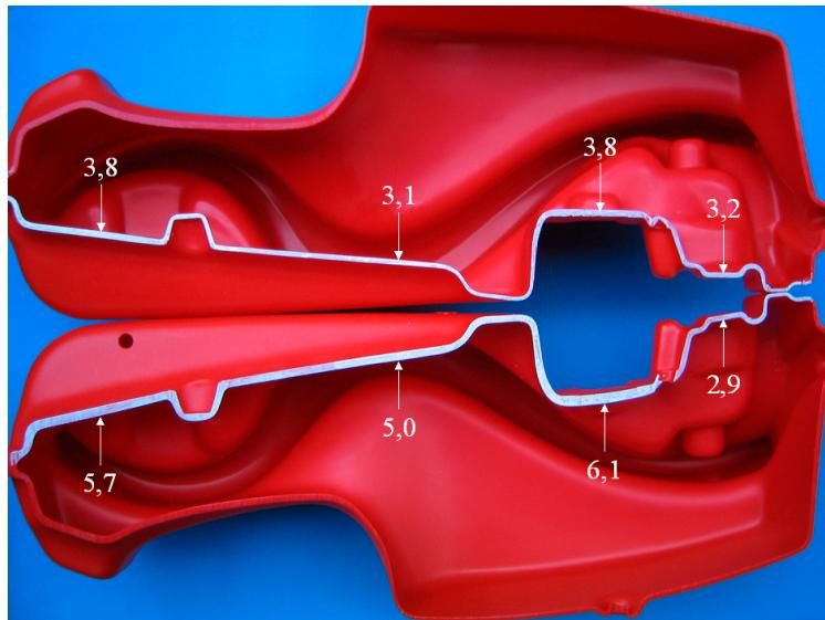
Fig. 6 Comparison of wall thickness distribution (in mm) in the bottom region of the blow moulded Bobby Car produced using a Flex Ring head (above) and a conventional head (below)
