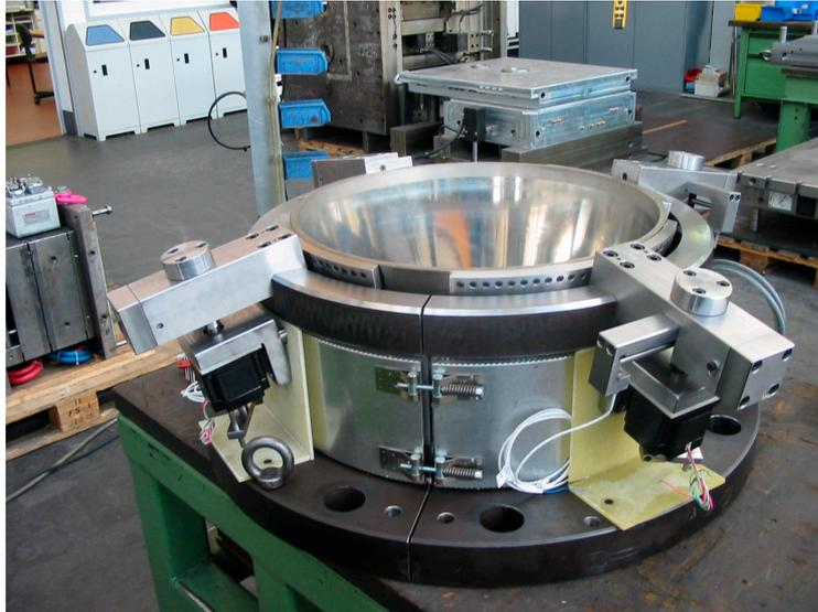
Fig. 8 Flex Ring assembly retrofitted into the head shown in Fig.7, having four adjusting pistons which act on special adjusting jaws
