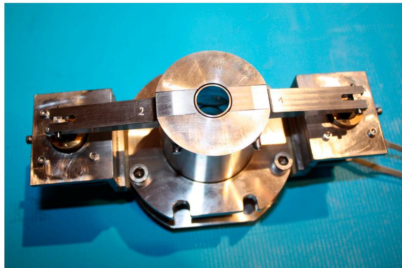
Fig. 3 Flex Ring unit to be retrofitted into a twelve cavity head for the production of an oval bottle having a volume of  $200 \text{ cm}^3$
