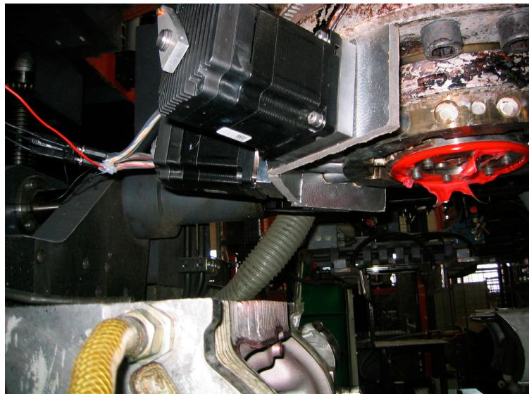
Fig. 5 Flex Ring solution for dynamic radial wall thickness control mounted to the production head
