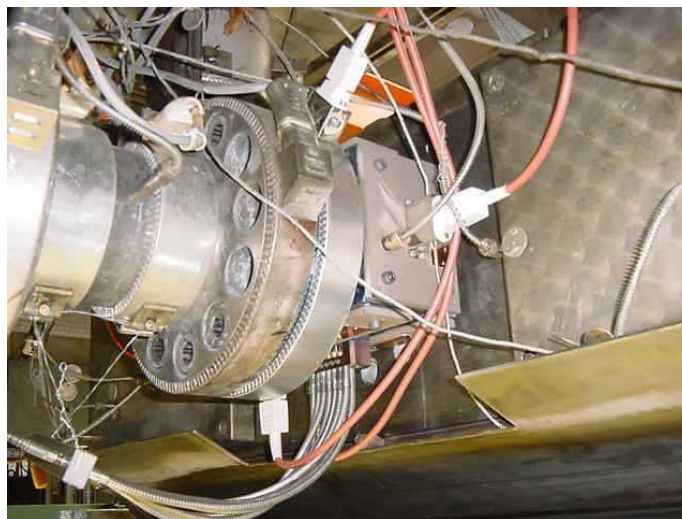
Fig. 9 Three-channel Membrane adapter (type ABA) mounted on a production line to cover a PC-sheet on both sides with a thin UV-protecting layer
