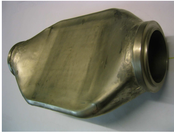
Fig. 13 Throttle body with the continuous transition from the central flat flow channel geometry to the respective circular inlet and outlet geometry
