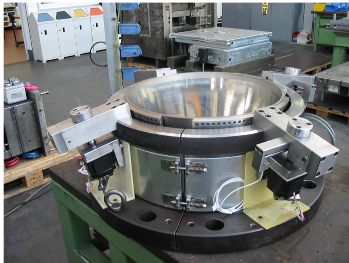
Fig. 5 Flexring die with a diameter of 550 mm having 20 single walls in the flexible conical area, which are dynamically deformed by four stepper drives while the parison is extracted
