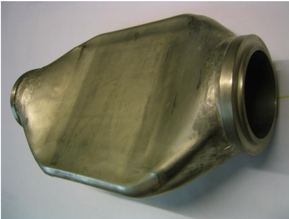
Fig. 7 Central flow channel piece of the throttle which has thick-walled solid flanges at both ends and is 20-walled in the whole middle region to give rise to a deformation
