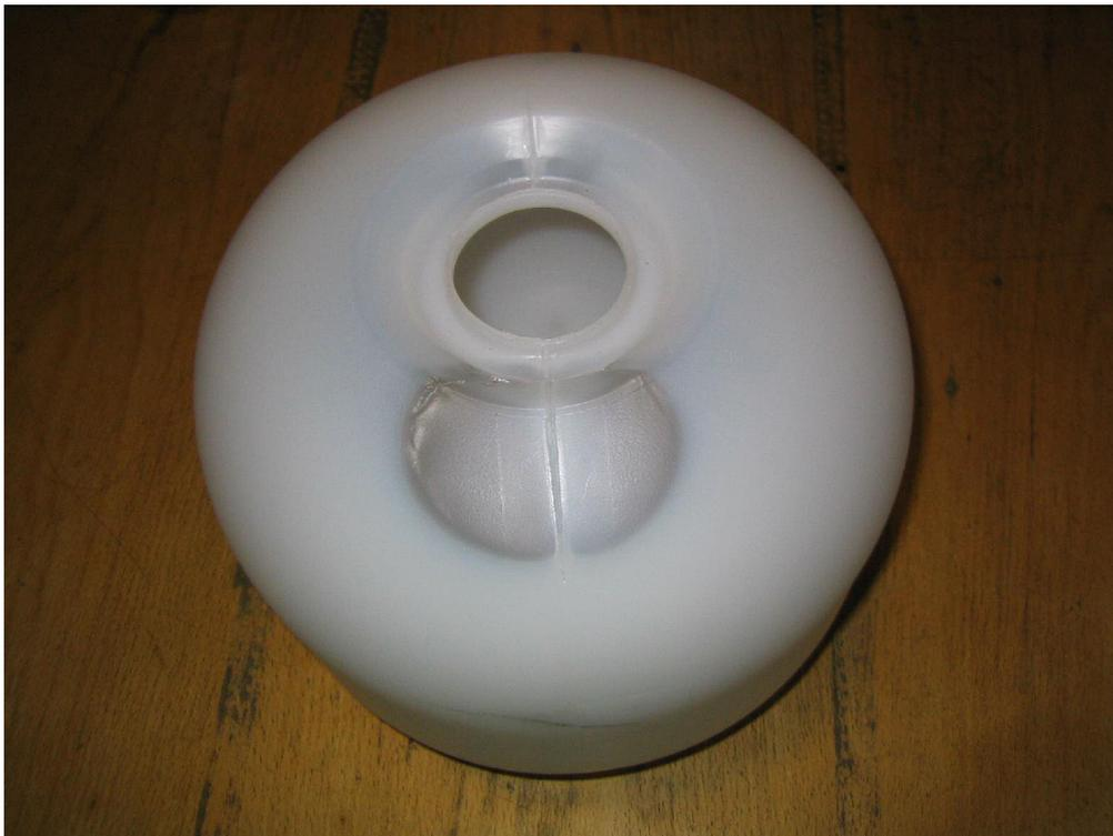
Fig. 4 Blow moulded bottle with extreme thin area which has been generated for the purposes of demonstration by short term local closure of the flow channel gap on the die by means of the setting jaw
