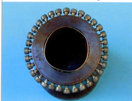
Figure 5: Enormous deformation of a 43 mm Flex Ring integrated into a test die for extrusion blow molding
